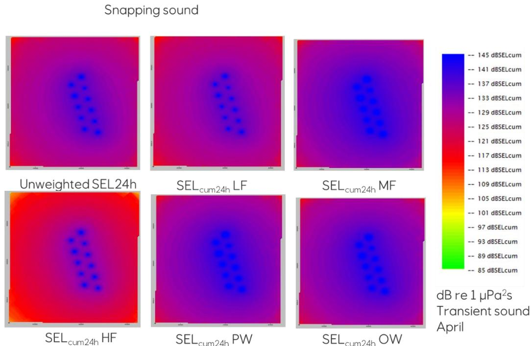
Fig 16. SELcum 24 of this transient sound as unweighted and weighted SEL<sub>cum24h</sub> shows that the threshold limits for injury are not exceeded at any distance to the wind turbines.
