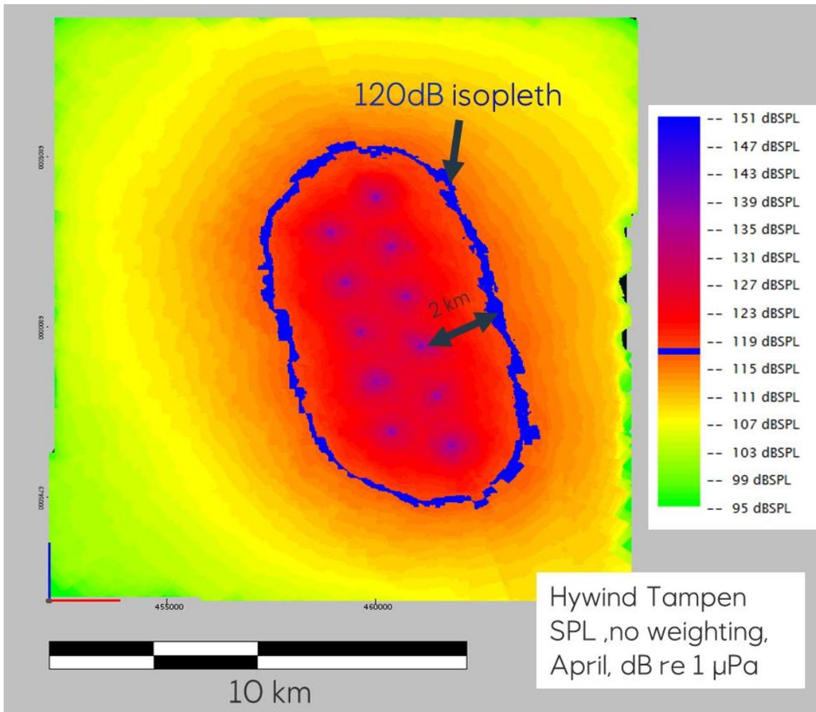
Fig. 13 Isopleth of the 120dB re 1  $\mu$ Pa threshold limit for behavioural disturbance (Table 4) around the Hywind Tampen windmills.
