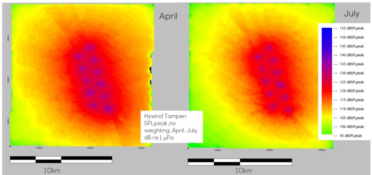
Fig. 11 Sound pressure levels SPLpeak for April and July simulation. Highest level from all depth projected to the surface.
