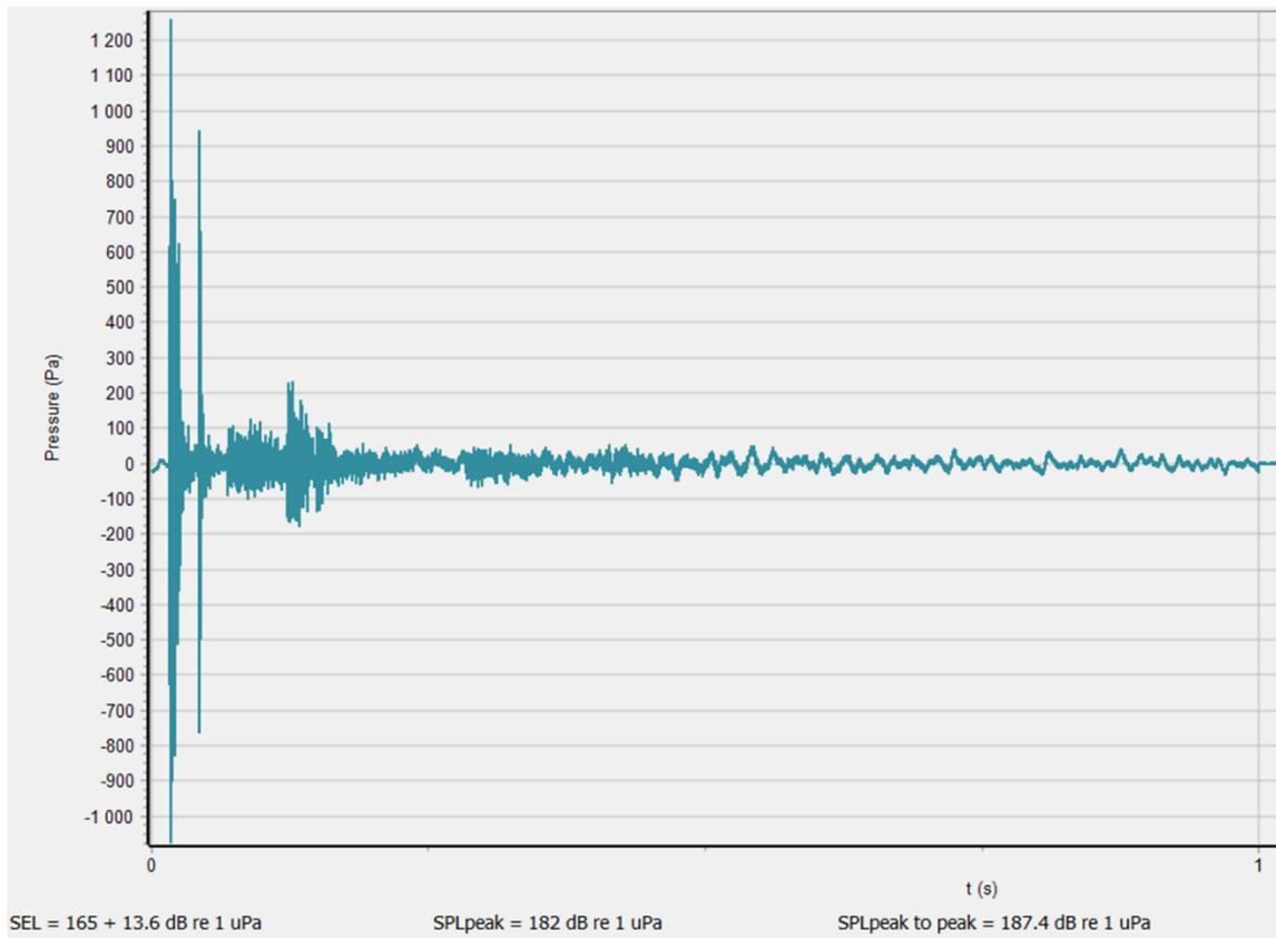
Fig 9. Input data for transient sound used in modelling software. Example for HY01. Original wav file measured at 150m distance upscaled to source level at 1 m from source.
