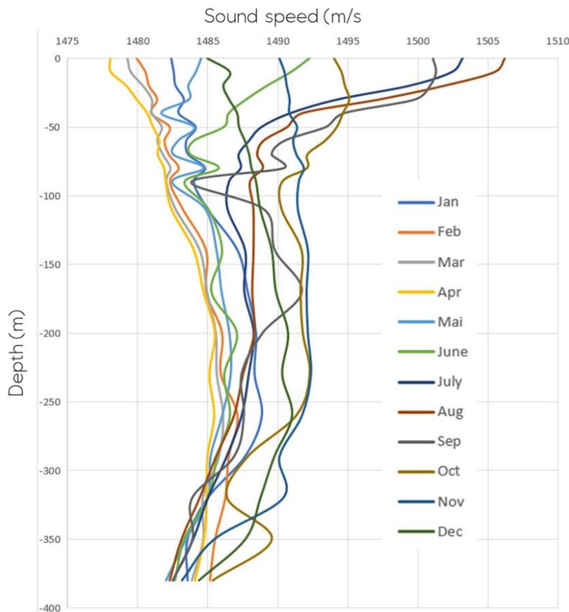
Fig 5. Sound speed profiles representative for the area for each month. For simulations sound speed profilrs form April and June were used.
