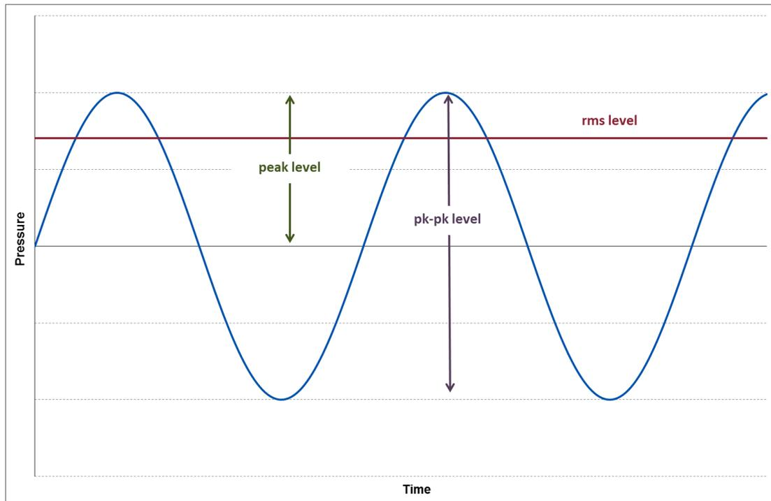
Fig. 2 Graphical representation of acoustic wave descriptors.
