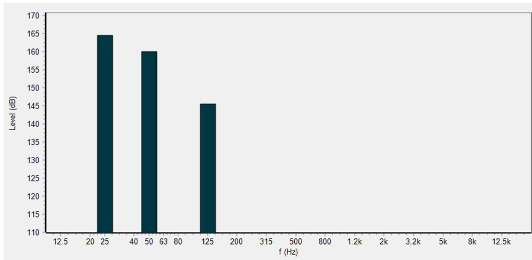
Fig. 7. Spectral content of the operational noise used in the sound simulations. Only those frequency bands that show clear difference to the general ambient sound in the area are shown.
