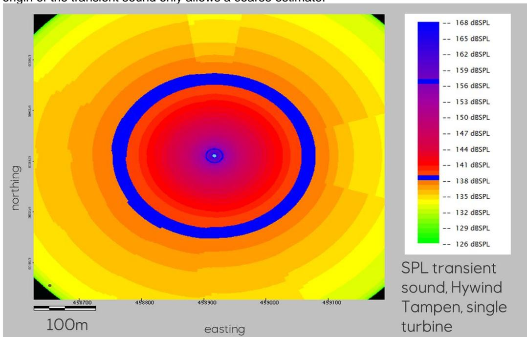
Fig. 15. SPL around a single turbine with indication of threshold limit for mild behavioural reaction to marine mammals. Average distance to the SPL 140 dB re 1  $\mu$ Pa isopleth is 160m, those to the SPL 160 dB re 1  $\mu$ Pa isopleth is about 8m.
