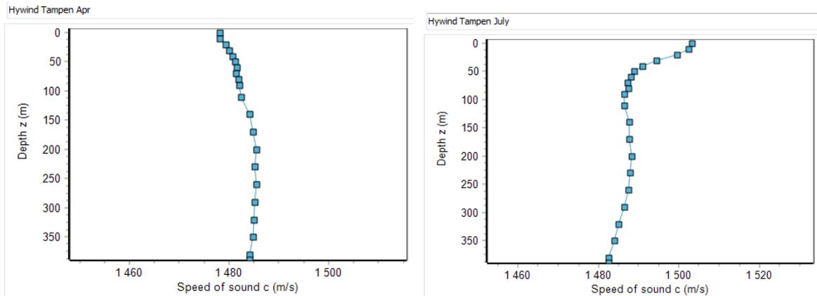
Fig 6. Sound speed profiles for April (left) and July (right) as used in dBSea
