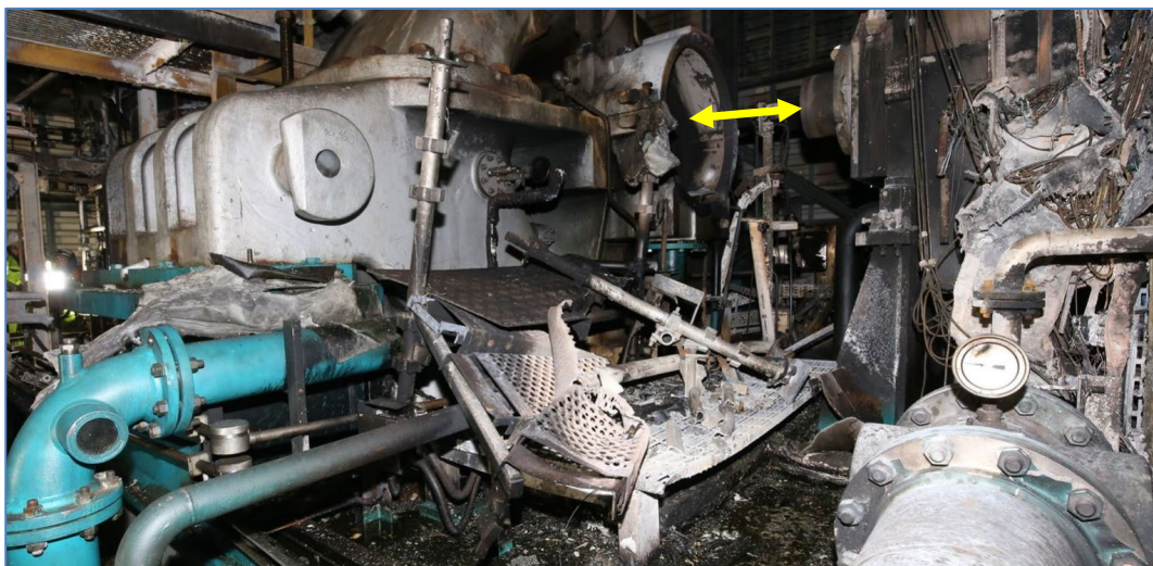
Figure 2-1 Turbine generator after the fire. The picture shows that the coupling between the steam turbine (left) and the gear (right) is missing
