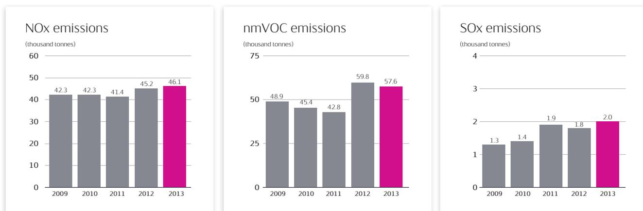
Nitrogen oxide (NO<sub>x</sub>) emissions from Statoil-operated assets increased from 45.2 thousand tonnes in 2012 to 46.1 thousand tonnes in 2013. The increase was mainly caused by an increase in exploration activities in 2013 compared with 2012 and an increase in the production from our US onshore operations.
