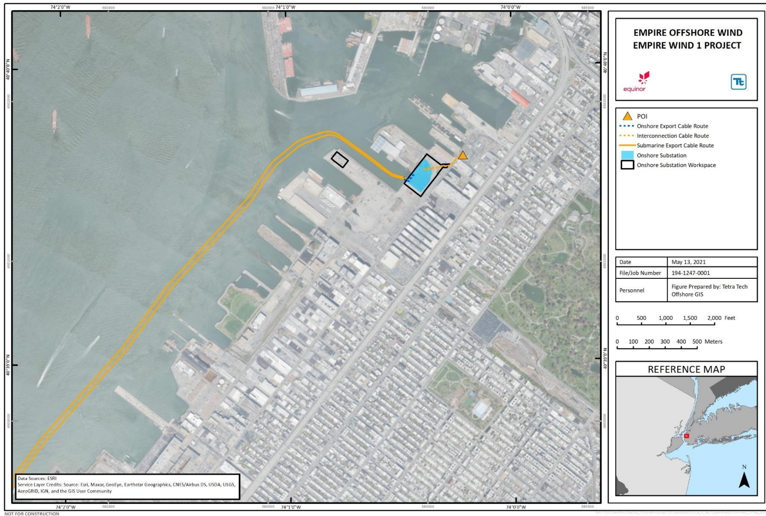
Figure 2. Overview of the submarine export cable route where it approaches the onshore substation, and the onshore interconnection cable route extending from the onshore substation to the proposed POI in Gowanus.
